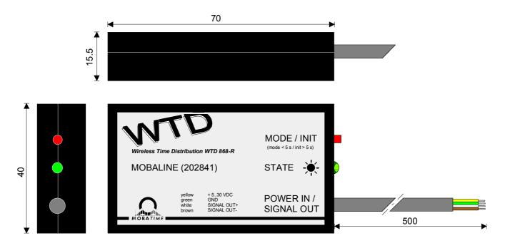
The interface can be installed directly on the device to be synchronised or up to 0.5 m displaced from said device using double-sided Velcro. The cable can be shortened or lengthened (cable  $4 \times 0.25 \text{ mm}^2$ ).
