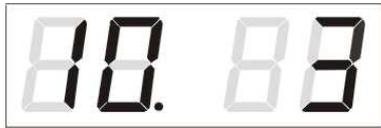
Enter the month in which the daylight saving time ends. Push **PB1S**. Enter the hour at which the daylight saving time ends.
