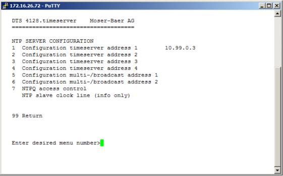
Path: 2 Configuration → 2 Time handling → 3 NTP server configuration
