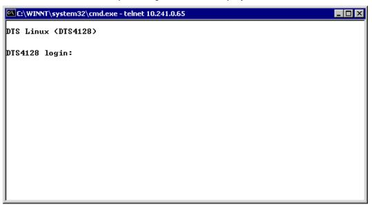
To start the menu, *dts* must be logged in as user. The standard password is *dts*. (Changing the password  $\rightarrow$  see Chapter "6.5.15 General Settings").
