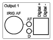
Each of the two lines has four output fields. Each output field carries the corresponding AF and digital signals.
