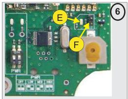
In "initialisation" mode, the LED (E) is on. To switch the repeater back in Init mode, short the two pins (F) for 3 seconds.
