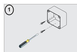
Mount the repeater in the area covered by the transmitter. Under no circumstances the transmitter should be directly mounted on a metallic surface.
