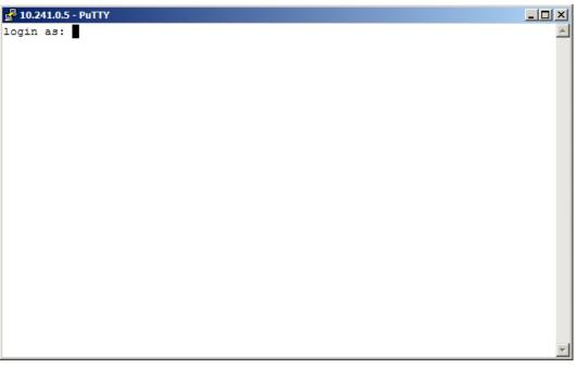
To start the menu, *dts* must be logged in as user. The standard password is *dts*. (Changing the password  $\rightarrow$  see chapter "6.5.20 General settings").
