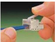
Pulled off spring terminal with operation tool: 2 operation tools are delivered with the accessory bag.
