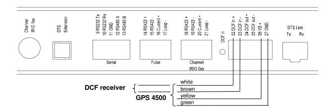
GNSS 3000 according to manual Bx-800813 chap. 9.2 Connection schematics DCF current
