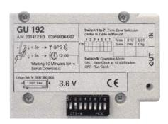
Time zone selectable by means of a DIP switches.
